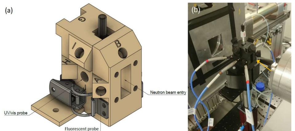
Fig 1. Two part quartz flow cell mount. 10 input ports enables multiple characterization techniques parallel to SANS measurements. Possible probes: UV/Vis, fluorescence, Raman, temperature readings and camera inspection etc.
