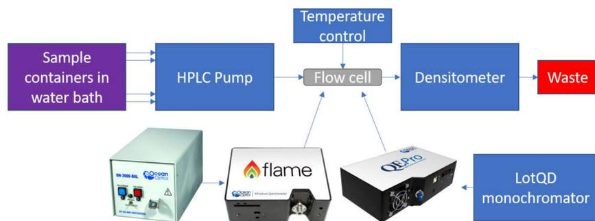
Fig 2. Schematic hardware setup. Sample delivered by HPLC pump to the flow cell, where SANS, UV and FL measurements are done. In-line densitometer provides additional data before sample is pumped to waste. Temperature control system is presented in Fig 3.
