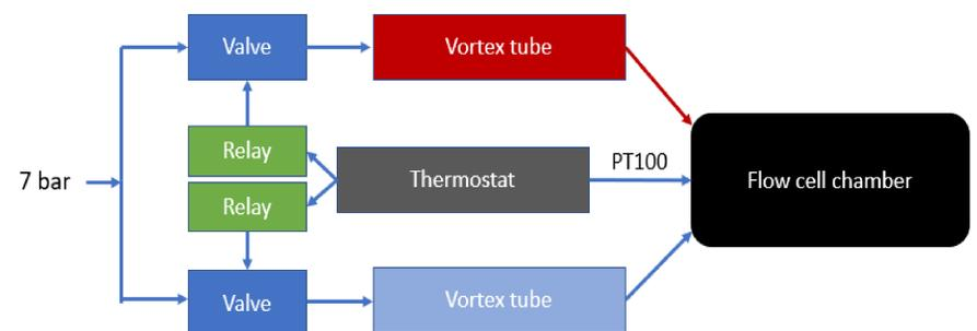
Fig 3. Schematic temperature control setup. Pressurized air flow is used to generate a hot and a cold air stream with the help of vortex tubes. Flow through the vortex tubes are controlled by solenoid valves. The air is lead into to flow cell chamber. Since pressurized air has a low moisture content, condensation on the flow cell is minimized.
