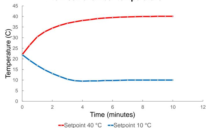
Fig 5. Temperature control capabilities. Set temperature is within 0.2 °C of setpoint after 7 minutes
