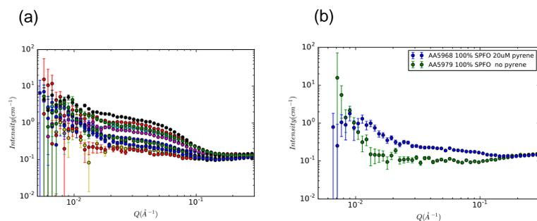
Fig. 4. SANS results measured at Zoom (ISIS facility, UK) for (a) a series of compositions from 100% Brij 35 to 100% sodium perfluorooctanoate (SPFO) at 5 mM in D<sub>2</sub>O and (b) comparison of SANS for the SPFO with and without pyrene (20 μM) showing that the fluorescent probe alters the micelles.
